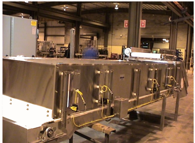
Bulk Storage Conveyor
