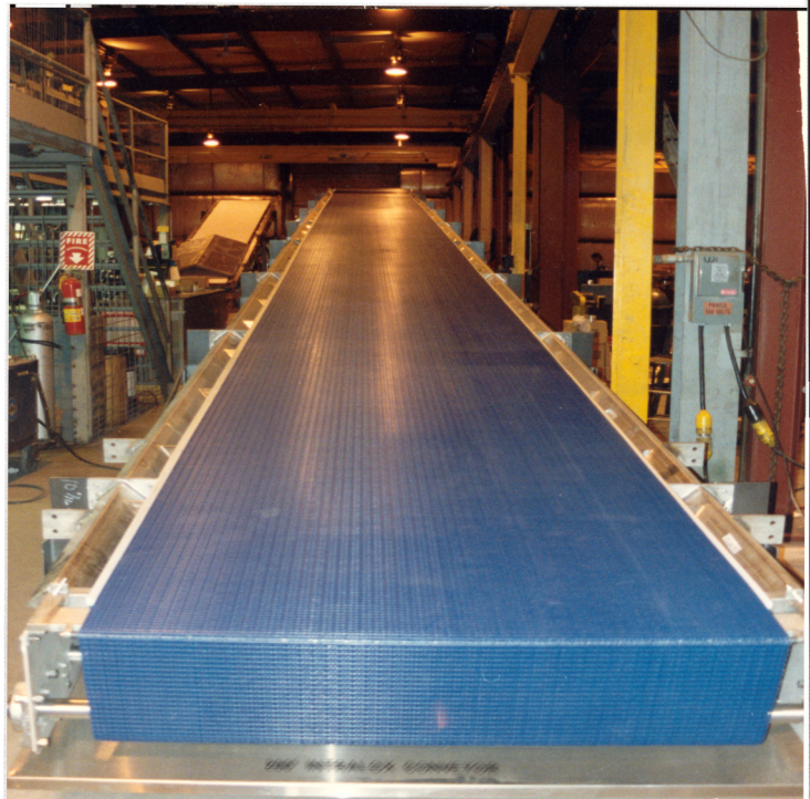
200' Snack Cooling Conveyor
